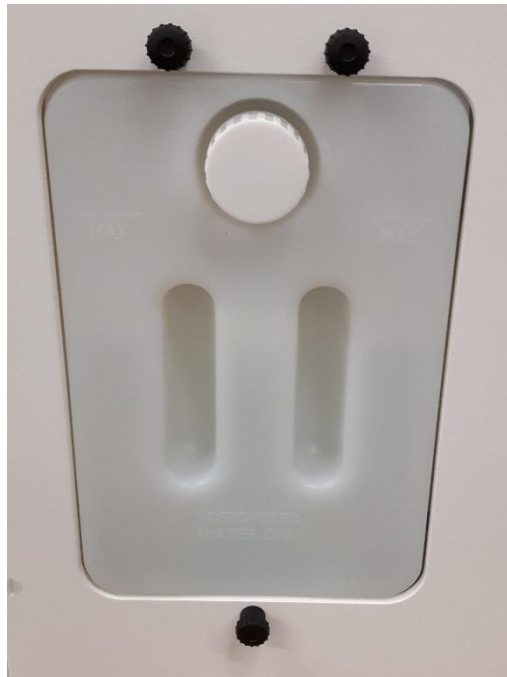
Figure 20: Humidity System Water Tank
