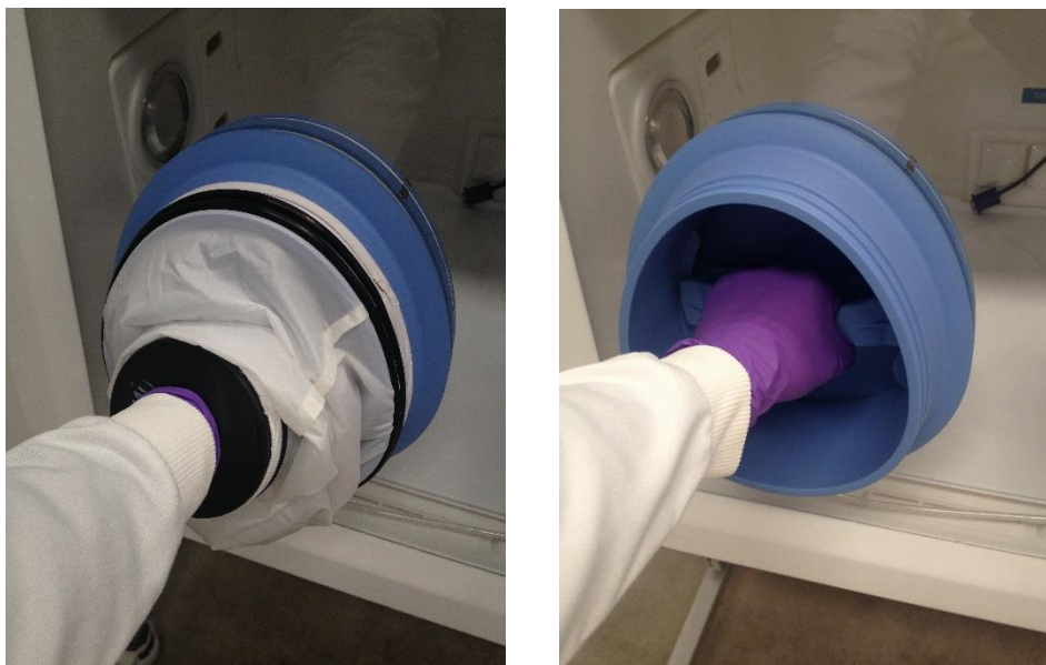
Figure 9: Arm inserted into Ezee-Sleeve (Shown with and without Ezee-Sleeve)
