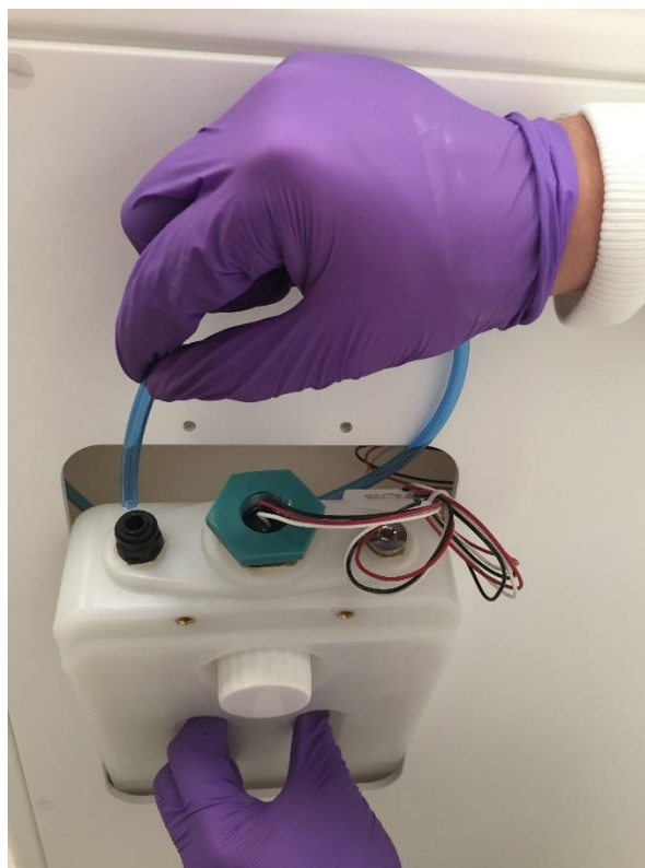
Figure 24: Water Tank top tube removal
