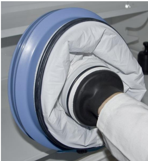
Figure 11: Ezee-Sleeve before vacuum
