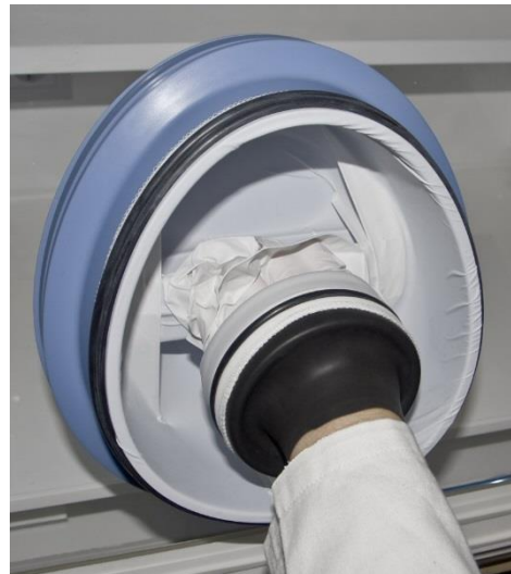
Figure 12: Ezee-Sleeve after vacuum
