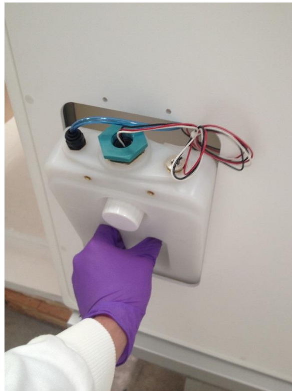
Figure 23: Water Tank tilted forward partially removed
