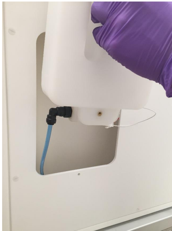
Figure 26: Water Tank bottom lifted out
